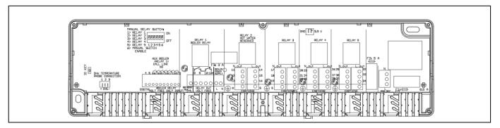
SMART ENERGY SWITCH is a central heating & colling wiring control center that fits most of the systems on the market in the Europe.
